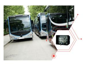
Our client, a bus manufacturer, has entrusted Viveris with the design and series production of a communication gateway between the CAN network and the IP network. This CAN/IP communication gateway provides access to the information from the vehicle's CAN bus to operational
